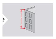
The result is shown in the main line and the measured distance above. Pressing the measuring key for 2 s in the function activates automatically Minimum or Maximum measurement.
