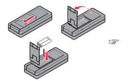
To ensure a reliable use, we recommend using high quality Alkaline batteries. Change batteries when battery symbol is flashing.
